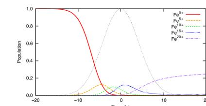
Population dynamics of Fe charge states during an XFEL pulse of 8 keV,  $5 \times 10^{12}$  photons/ $\mu\text{m}^2$ , 10 fs FWHM
