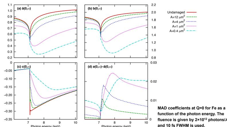
MAD coefficients at  $\mathbf{Q}=0$  for Fe as a function of the photon energy. The fluence is given by  $2 \times 10^{12}$  photons/ $\text{\AA}^2$  and 10 fs FWHM is used.
